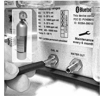
Carefully open the valve on the pressure gauge of the test gas bottle and set the required test pressure (see **Actual value**).
