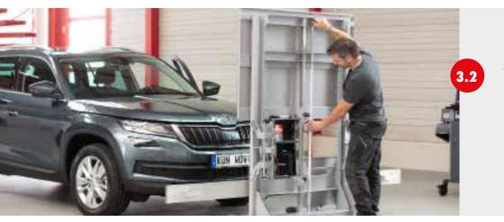
Adjustment of the calibration board holder for camera calibration by means of spring balancing. Possible up to 1.85 m and also suitable for vans.
