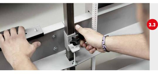
Adjustment of the laser carrier for radar calibration (up to 1.0 m).
