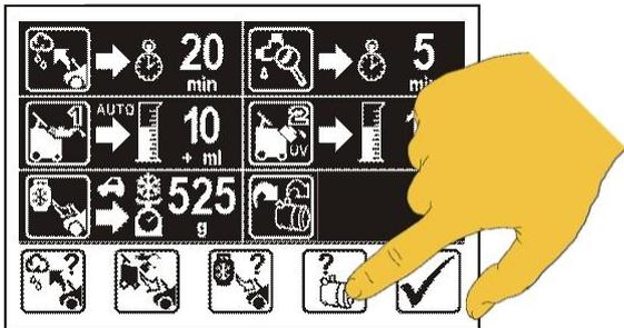
**Step 20** - Select the desired A/C charging side port for refrigerant charge.
