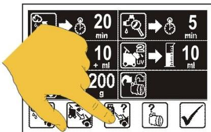
**Step 17** - To set the refrigerant weight touch the weight icon, or refrigerant charge weight can be selected by using database (touch car icon).
