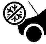
There is no refrigerant in the air-conditioning system or quick couplers not open.
