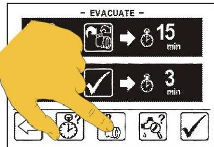
**Step 5** Select the desired A/C service port or ports. Evacuation process is more efficient when both suction and discharge ports are selected.
