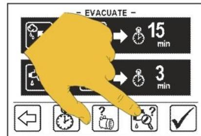
**Step 7 - Touch confirm icon if you want to select leak test, touch X icon to abort leak test under vacuum.**
